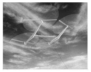
Fig -4: Four rotor demonstration craft
