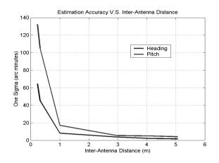
Chart -1: Relationship between the achievable GPS-derived heading and pitch accuracy
