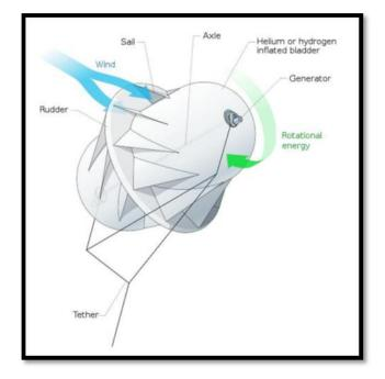
**Fig -2**: Construction of a FEG
